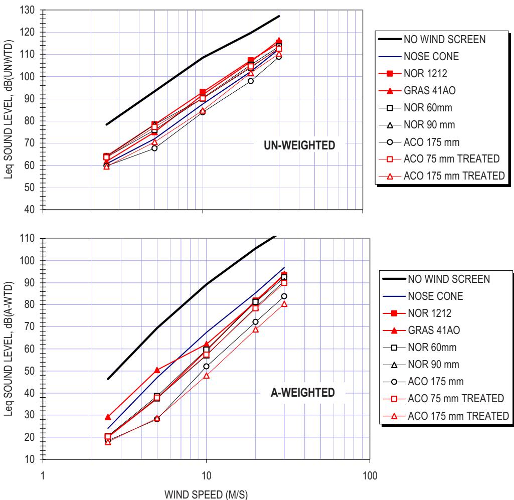
*Fig. 6—Plot of overall flow noise response for windscreen models. Upper: Un-weighted level, Lower: A-weighted level.*
